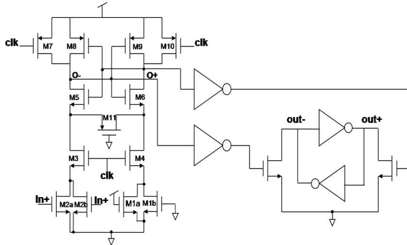
Fig. 5: Self Referenced Modified Poulton-Dally-Tell sampler(SRMPDT)
