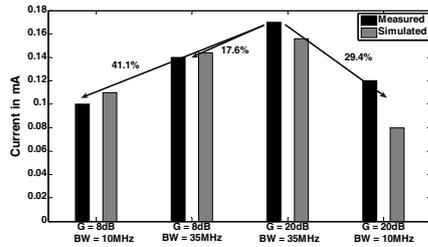
Fig. 9. Measured Current Consumption and Savings for VGBWA
