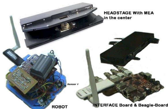
Fig. 3. Headstage, Interface board and the robot
