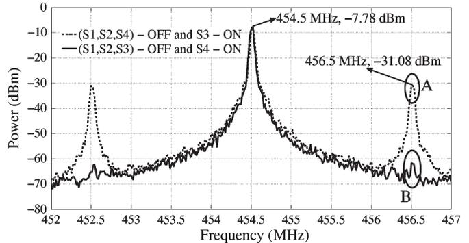
Fig. 7. VCO output spectrum (open loop) with spurs at an offset of 2 MHz in response to the 2-MHz noise injected into the substrate.
