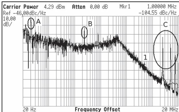
Fig. 5. Measured phase noise characteristics of a 500-MHz signal with spurs at an offset of 5 MHz generated due to the periodic substrate noise.
