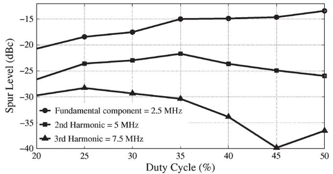
Fig. 11. Effect of the harmonic components of a pulsed clock on PLL output spurious tones.
