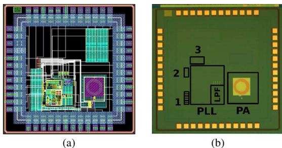
Fig. 6. Location of the noise injector buffers (1, 2, 3) and the PLL. (a) Chip layout. (b) Die.
