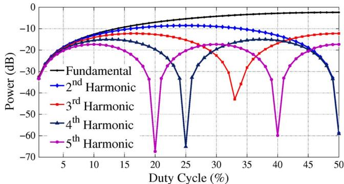
Fig. 2. Harmonic content of a 10-MHz clock signal as a function of its duty cycle.
