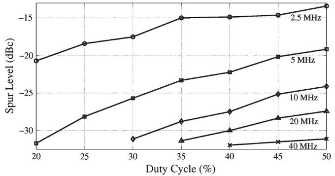
Fig. 10. Measured sensitivity of the PLL output spur level to the frequency and the duty cycle of the periodic substrate noise.
