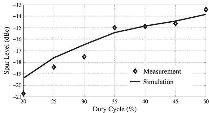
Fig. 12. Simulation and measured results of the sensitivity of the PLL output spur level to the duty cycle of the periodic substrate noise of 2.5 MHz.
