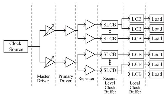
Fig. 1. Clock distribution network using a multilevel tree architecture used in synchronous digital systems.
