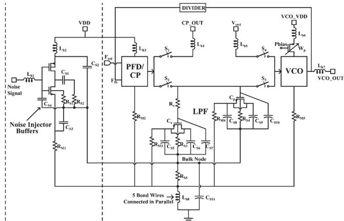
Fig. 3. Test bench. Type-II third-order integer-N CP PLL and noise injector buffers.
