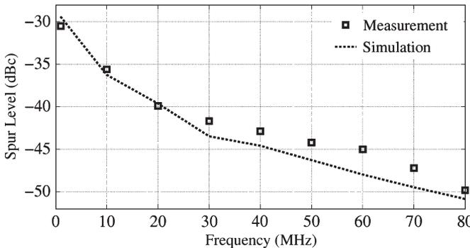
Fig. 9. Sensitivity of the VCO (open loop) output spur level to the periodic noise frequency.
