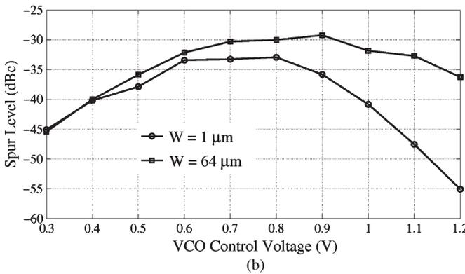
Fig. 8. Open-loop VCO characterization. (a) Sensitivity of the VCO gain to control voltage. (b) Spur-level dependence on the VCO control voltage.
