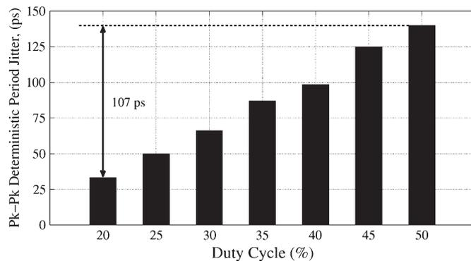
Fig. 13. Measured duty cycle effects of the 5-MHz noise injected into the substrate on the Pk-Pk deterministic period jitter.
