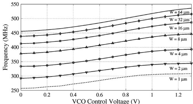
Fig. 4. Measured VCO transfer characteristics with different bias-current transistor widths  $W_p$ .
