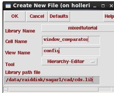
Figure 6: Config view for the mixed mode schematic
