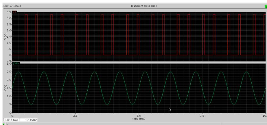
Figure 9: Window comparator detects when Vin is between 1 and 1.5v
