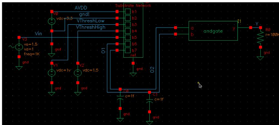
Figure 5: Completed window comparator schematic with test voltage sources
