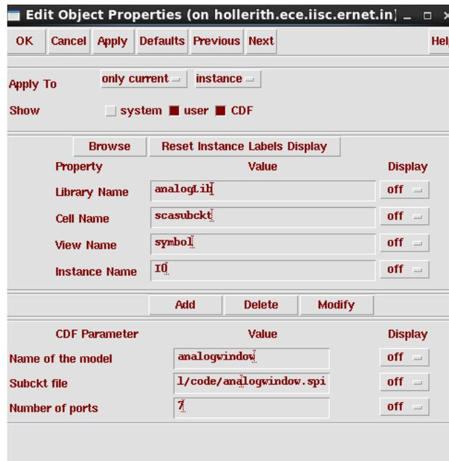
Figure 4: Instantiating a SPICE netlist in the schematic
