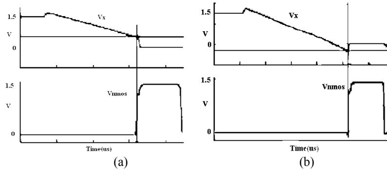
**Fig 5:** a) Dead time too short: Capacitive Switching loss, b) Dead time too long, body diode losses.
