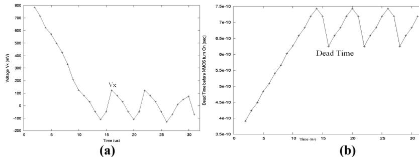
**Fig. 7: a)** Value of  $V_x$  when NMOS turns On for dynamic loads of  $800\Omega$  and  $400\Omega$  . **b)** Variation in dead time for NMOS turn On with time.
