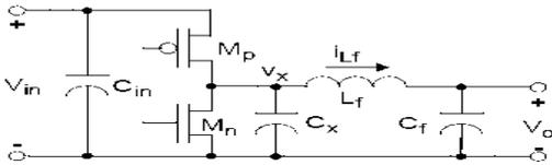
**Fig. 1:** A DC-DC buck converter
