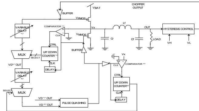
**Fig. 3:** Proposed Buck Converter with PFM control and adaptive ZVS scheme
