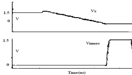
**Fig 6:** Adaptive dead time control to implement ZVS for NMOS turn ON.
