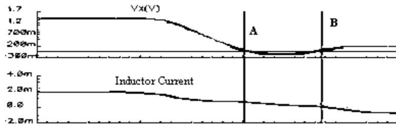
Fig. 2: Minimum duration for Inductor current reversal
