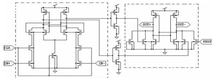
**Fig 4:** Clocked comparator (*Vijay and Amrutur (2007)*).
