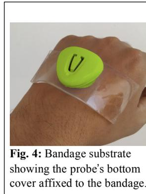
**Fig. 4:** Bandage substrate showing the probe's bottom cover affixed to the bandage.
