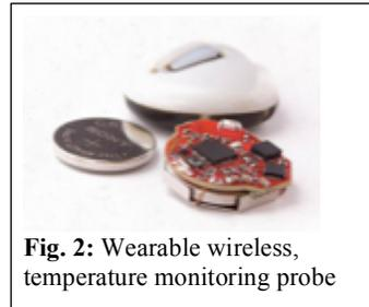
**Fig. 2:** Wearable wireless, temperature monitoring probe
