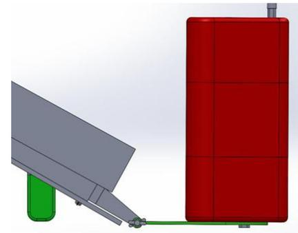
Figure 4: Ultrasonic sensor module (green) and Quality sensor module (red)
