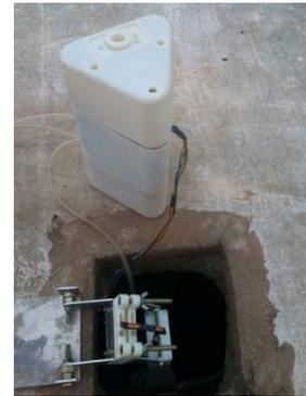
Figure 6: Integrated water level and water quality module deployed in a ground level reservoir. The level sensor unit is looking into the tank and is separate from the main controller module (white triangular box).
