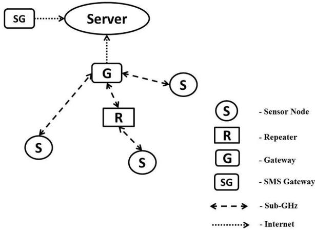
Figure 5: System Architecture consisting of the sensor nodes and gateway. These are connected in the star topology by wireless links.
