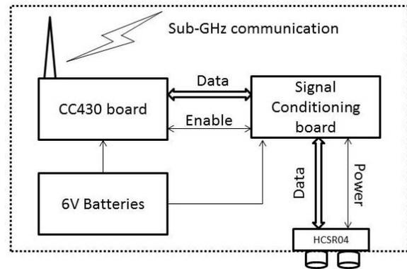
Figure 2: Sensor device architecture consisting of a microcontroller board based on TI's CC430 and a separate, power controlled, sensor signal conditioning board.
