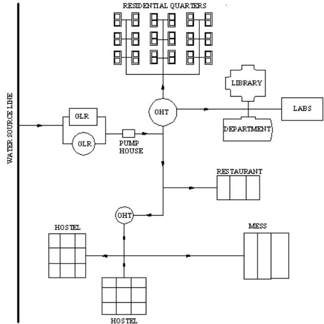
Figure 1: Schematic of a typical campus water network indicating intermediate storage reservoirs (GLR), overhead tanks (OHT) and the final consumers (buildings).
