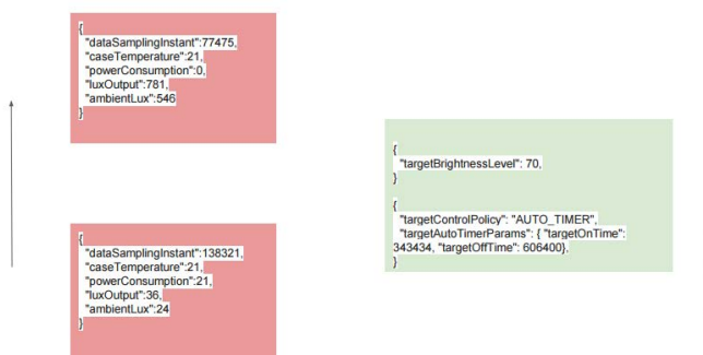
Figure 3: Street Light Observation and Control Data
