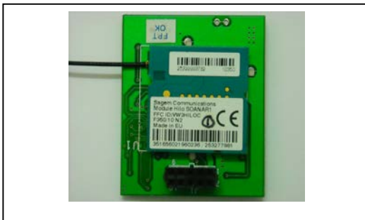
Fig.2b. communication module Board
