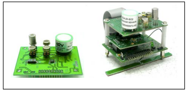
Fig.2c. Photograph of Sensor module and integrated board
