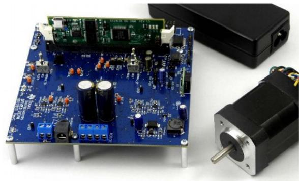
Figure 8. DRV8312, F2805x and BLDC motor.
