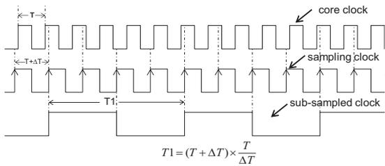
Figure 1. Illustration of sub-sampling system.
