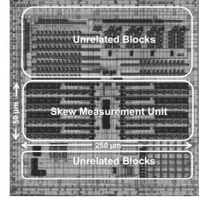
Figure 4. Chip layout of the skew measurement unit in 65nm CMOS Process.
