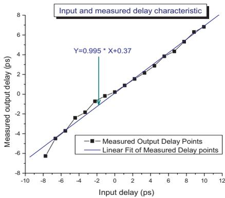
Figure 7. Input output delay characteristics.
