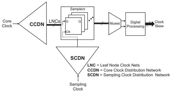
Figure 2. Illustration of the concept of skew measurement in a distributed clock network.
